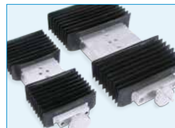
Way Covers – protect the slider and dovetail base from dust, dirt and grit that could hamper the efficient operation of the slide. Way covers increase slider height and reduce the travel length of linear UniSlides.
